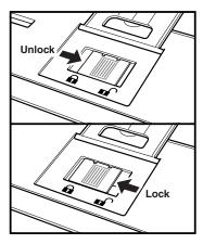
The scanner mechanism inside the scanner unit is locked to avoid movement during transport. Before setting the DR-2580C on the scanner unit, be sure to unlock the scanning unit slide lock.
