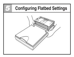
Whenever moving the scanner unit, grip it with both hands to keep it from falling. The scanner unit weighs approximately 8.4lb (3.8 kg) alone, while the DR-2580C and scanner unit together weigh approximately 12.6 lb (5.7 kg).
