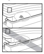
Positioning the DR-2580C on its protrusions to enter the holes in the bottom of the DR-2580C ①, and then slide the scanner unit forward into place ②.
