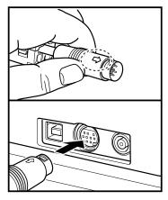
Making sure the arrow on the plug is on top, insert the plug into the connector as far as it will go.
