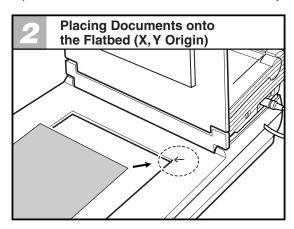
The upper right corner of the flatbed (platen glass) is the origin (0, 0) of the X, Y coordinates.
