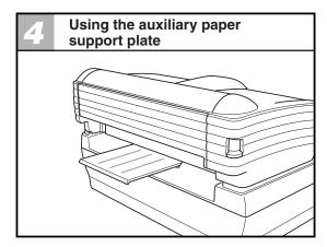
Extend the auxiliary paper support plate on the back of the scanner unit when performing Straight Path scanning with the DR-2580C. Pulling out the auxiliary paper support plate when cards and other originals are output during Straight Path scanning will keep the output documents from falling from the scanner unit.
