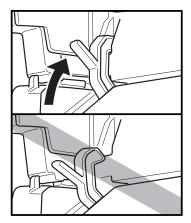
Check to make sure that the DR-2580C is not loose, and that the hooks on the left and right of the scanner unit secure the DR-2580C in place. Check to make sure that the hooks are fully engaged.
